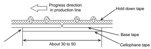
No lifting for the direction of progressing
