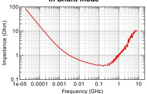
Figure 2 - 100nF ULSC Measured results (module of Z-parameters)
