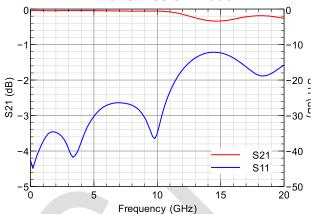
Figure 3 - 100nF ULSC measurement results (module of parameters)
