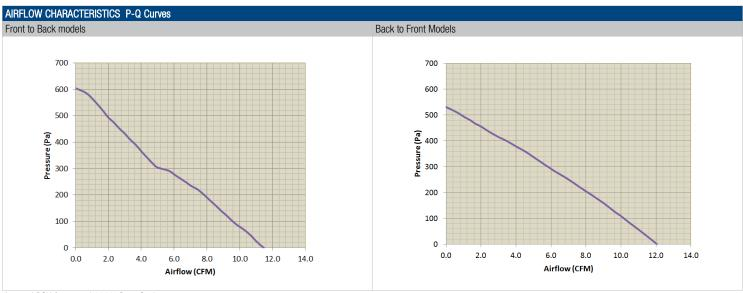
Internal PSU fan speed 100% Duty Cycle
