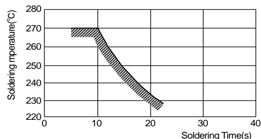
[Allowable Flow Soldering Temperature and Time]
