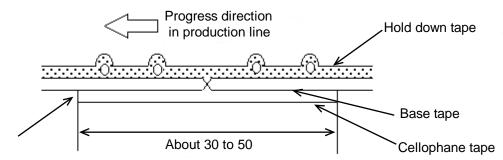
No lifting for the direction of progressing
