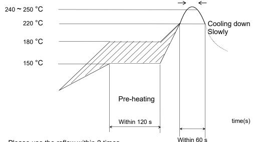
Please use the reflow within 2 times. Within 60 s Use rosin type flux or weakly active flux with a chlorine content of 0.2 wt % or less.
