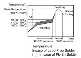
[Allowable Reflow Soldering Temperature and Time]
