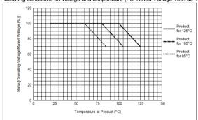
Derated products\*1 are suitable for use in circuits where continuous applied voltage and temperature to the capacitor is derated (below rated voltage and temperature).
