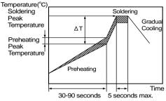
[Allowable Flow Soldering Temperature and Time]
