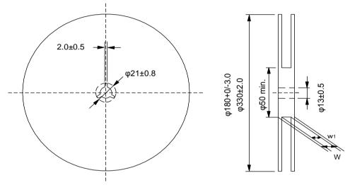
Fig.3 Taping Diagram
