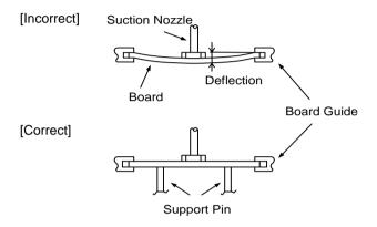
2.Dirt particles and dust accumulated in the suction nozzle and suction mechanism prevent the nozzle from moving smoothly. This creates excessive force on the capacitor during mounting, causing cracked chips. Also, the locating claw, when worn out, imposes uneven forces on the chip when positioning, causing cracked chips. The suction nozzle and the locating claw must be maintained, checked and replaced periodically.
