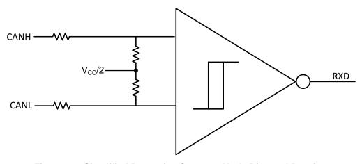
Figure 26. Simplified Recessive Common Mode Bias and Receiver
