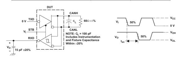
Figure 17. Ten Test Circuit and Voltage Waveforms
