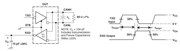
All  $V_I$  input pulses are from 0 V to  $V_{CC}$  and supplied by a generator with the following characteristics:  $t_r$  or  $t_f \le 6$  ns. Pulse Repetition Rate (PRR) = 125 kHz, 50% duty cycle.
