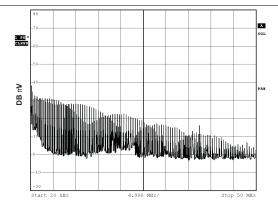
Figure 9. Frequency Spectrum of Common-Mode Emissions
