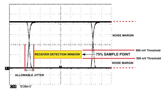
Figure 30. Typical CAN Differential Signal Eye-Pattern
