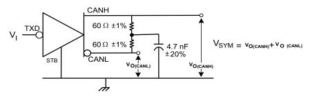
Figure 23. Driver Output Symmetry Test Circuit
