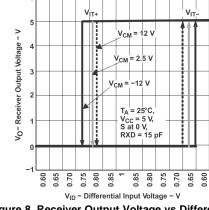
Figure 8. Receiver Output Voltage vs Differential Input Voltage
