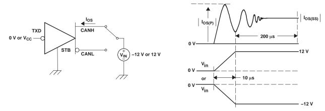
Figure 22. Driver Short-Circuit Current Test and Waveform
