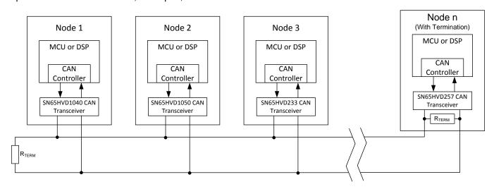
Figure 28. Typical CAN Bus
