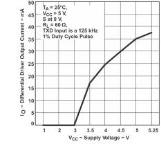
Figure 7. Driver Output Current vs Supply Voltage
