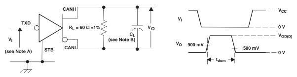
All V<sub>I</sub> input pulses are from 0 V to V<sub>CC</sub> and supplied by a generator with the following characteristics:  $t_r$  or  $t_f \le 6$  ns. Pulse Repetition Rate (PRR) = 500 Hz, 50% duty cycle.
