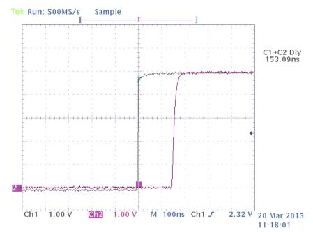
Figure 33.  $t_{loop}$  Delay Waveform
