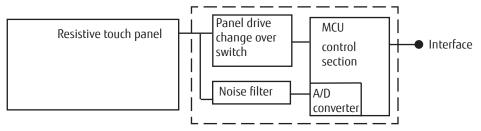
Resistive touch panel controller chip or board
