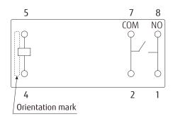
Connect terminal #1 and #8 on the PC board
