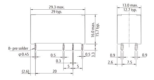
Note: Dimensions of the terminals do not include thickness of pre-solder. Dimensions do not include tolerance.
