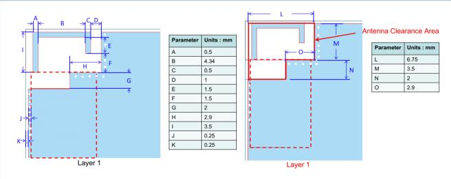
Fig 13. QN9080-001-M17 module on 36 mm x 31 mm GND PCB layout guide - corner - clearance area layer 1 dimensions
