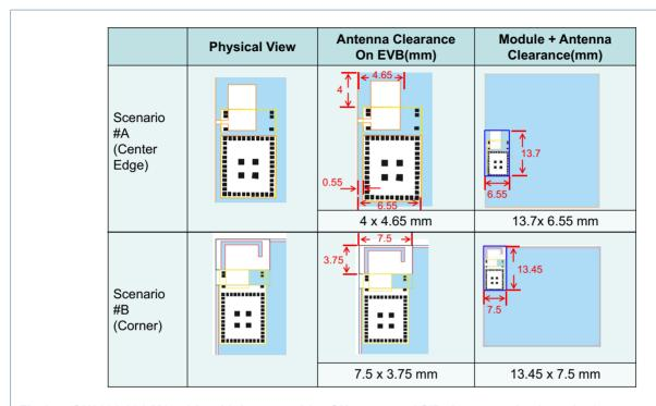
Fig 6. QN9080-001-M17 chip with integrated 2.4 GHz antenna / SIP clearance size (top view)
