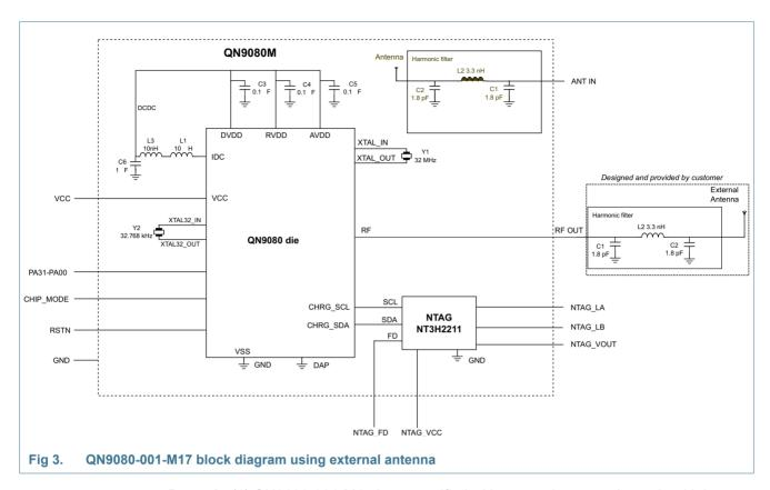
**Remark:** (1) QN9080-001-M17 is not certified with external antenna but only with its internal antenna. Customer using external antenna has to do new certification. (2) Harmonic filter is in adequacy with board.
