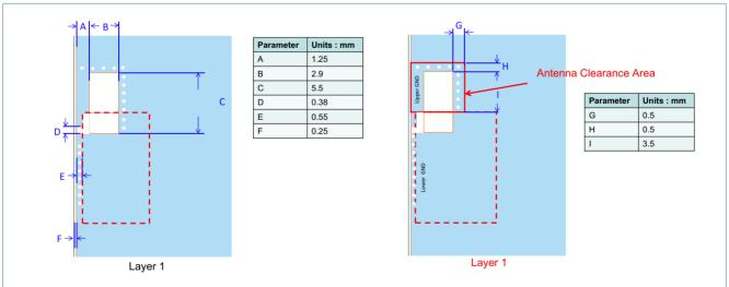
Fig 9. QN9080-001-M17 module on 36 mm x 31 mm GND PCB layout guide - center edge - clearance area layer 1 dimensions
