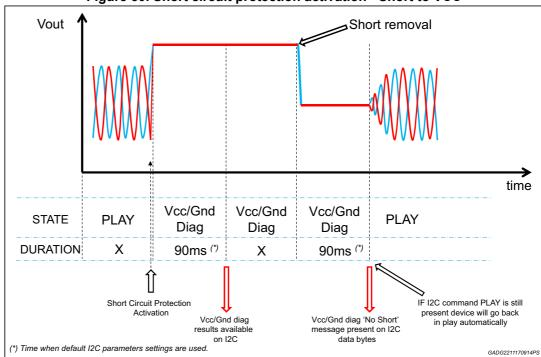
Figure 50. Short circuit protection activation - Short to VCC
