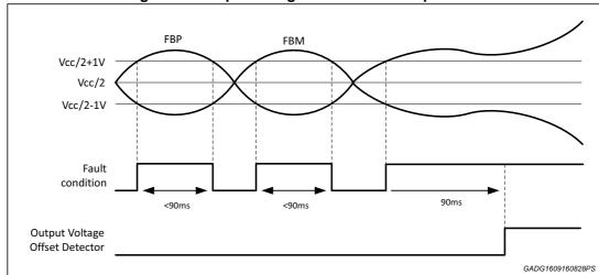
Figure 55. Output voltage offset detector operation
