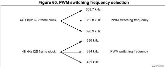
Actually, the PWM spectrum of the output square wave can be controlled in AM band just in case it is possible to fix the switching frequency, in other words without skipping any power stage commutation (typical phenomenon for a class D amplifier close to the clipping). The device provides an additional function called LRF (Low Radiation Function). This I<sup>2</sup>C option assures a minimum duty cycle for the PWM output square wave avoiding any missing pulses.
