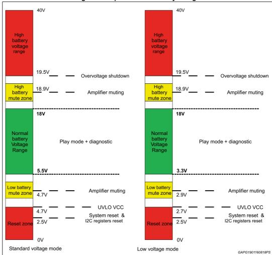
Figure 39. Operation vs. battery charge
