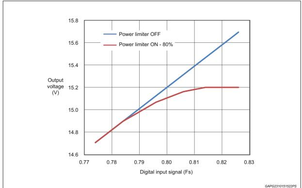
Figure 45. Response obtained with a limitation corresponding to 80% of the full-scale
