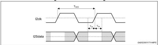
Figure 68. I<sup>2</sup>S clock transition timings
