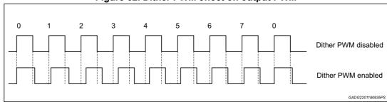
Figure 62. Dither PWM effect on output PWM
