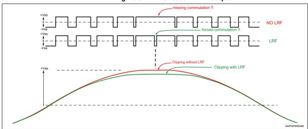
Figure 61. LRF effect on PWM output
