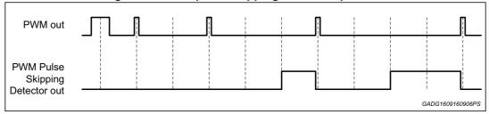
In order to enable the PWM pulse skipping detector, the user must set IB5[5,4]='01'.
