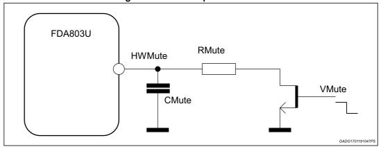
Figure 44. HWMute pin schematic
