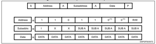
1. The I<sup>2</sup>C addresses are: Address 1 = 1110000 Address 2 = 1110001 Address 3 = 1110010 Address 4 = 1110011
