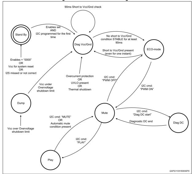
Figure 38. Finite state machine diagram
