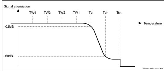
Figure 59. Thermal attenuation curve
