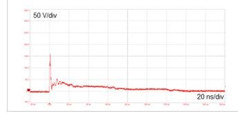
Figure 5. ESD response to ISO 10605 - C = 150 pF, R =  $330 \Omega$  (-8 kV contact discharge)
