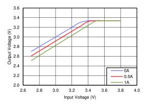
Figure 7-6. Typical Dropout Behavior, V<sub>OUT</sub> = 3.3 V
