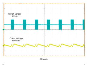
Figure 7-8. Typical PFM Mode Waveforms:  $V_{IN}$  = 3.6 V,  $V_{OUT}$  = 1.8 V,  $I_{OUT}$  = 10 mA
