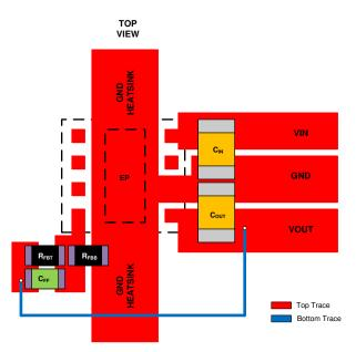
Figure 10-2. Example PCB Layout
