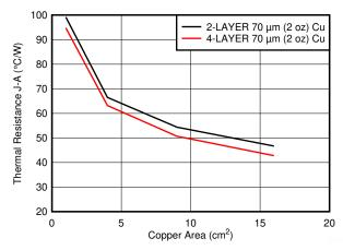
Figure 8-3.  $R_{\theta JA}$  Versus Copper Board Area
