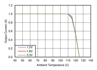
Figure 8-4. Maximum Output Current Versus Ambient Temperature, R<sub>0JA</sub> = 44°C/W, V<sub>IN</sub> = 5 V
