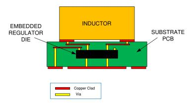
Figure 7-2. Package Side View Drawing
