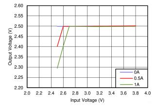
Figure 7-5. Typical Dropout Behavior, V<sub>OUT</sub> = 2.5 V
