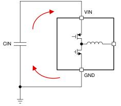
Figure 10-1. Current Loops With Fast Transient Currents
