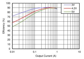
Typical Efficiency for V<sub>OUT</sub> = 1.8 V Auto Mode
