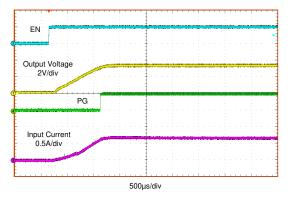
Figure 7-4. Typical Start-Up Waveforms, V<sub>IN</sub> = 5 V, V<sub>OUT</sub> = 3.3 V, I<sub>OUT</sub> = 1 A
