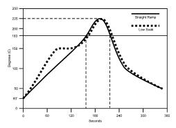
Figure 10-3. Typical Re-flow Profile Eutectic (63sn/37pb) Solder Paste
