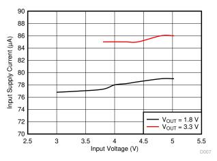
Figure 7-9. Typical No Load Input Supply Current
