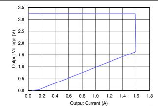
Figure 7-3. Typical Current Limit Profile V<sub>IN</sub> = 5 V, V<sub>OUT</sub> = 3.3 V
