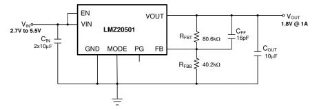
Figure 8-1. LMZ20501 Typical Application V<sub>OUT</sub> = 1.8 V
