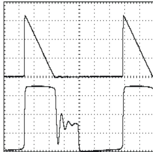
Channel-1 (Upper): I_{LED} @ 100mA/cm Channel-2 (Lower): V_{OUT} @ 1V/cm Timebase: 500ns/cm Operating Waveform for L = 6.8\mu H , V_{CC} = 1.5V
