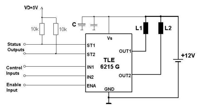
The blocking capacitor C is recommended to avoid critical negative voltage spikes on  $V_{\!s}$  in case of battery interruption during OFF-commutation.
