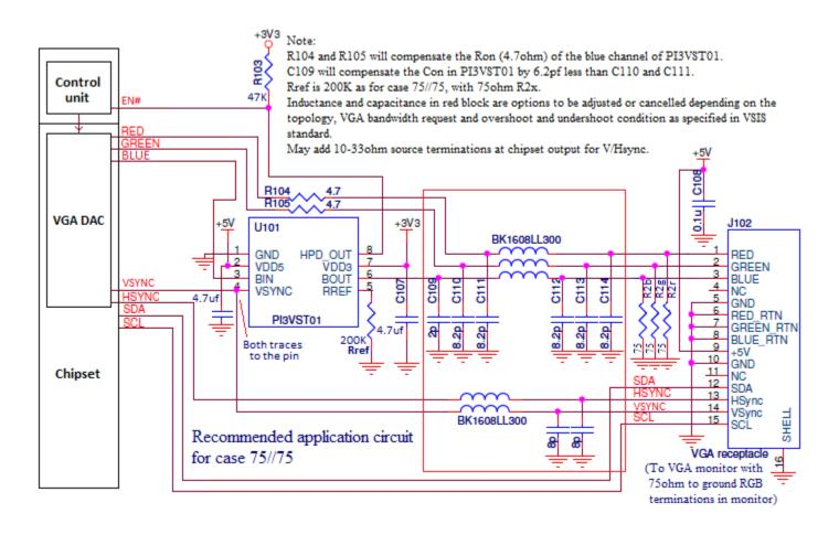
Total power dissipation of this solution is very small. PI3VST01 power dissipation is 0.66 mW typical, which is a small fraction (<1%) of the 170 mW saved when the monitor is not connected.
