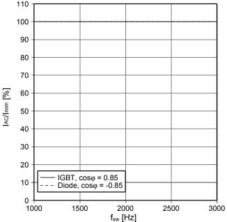
$$\begin{split} &T_{\text{inlet}} \text{- derating curve IGBT (motor), Diode (generator)} \\ &V_{\text{DC}} = 650 \text{ V}, \text{ V}_{\text{AC}} = 400 \text{ V}_{\text{RMS}}, f_{\text{AC sine}} = 50 \text{ Hz, } \cos\phi = \pm 0.85, \\ &T_{\text{inlet}} = 40 \text{ °C and nom. cooling conditions} \end{split}$$
