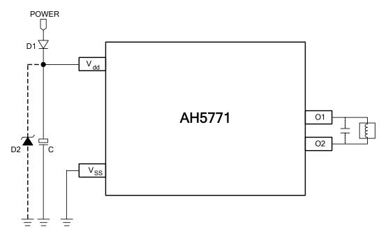
Note: D2 (Zenor Diode) and Capacitor C are for power stabilization, D2 is recommended to be 18Vz (option), C is recommended to  $0.1 \text{uF} \sim 1 \text{uF}$  (E-Cap). D1 (reverse Diode) is for reverse voltage protection.
