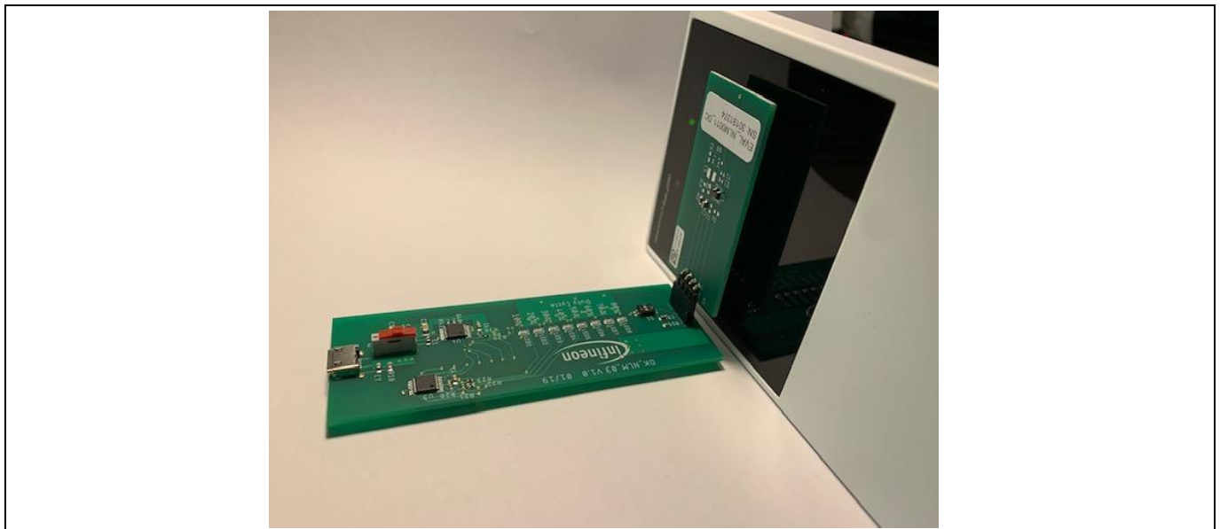
Figure 16 Connected boards placed reader antenna parallel to board antenna
