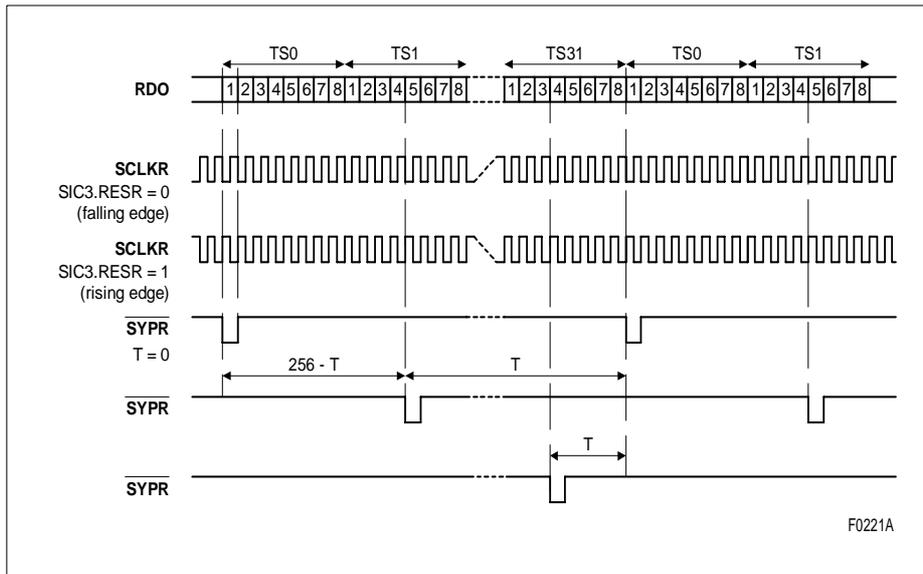
Figure 27 SYPR Offset Programming (2.048 Mbit/s, 2.048 MHz)
