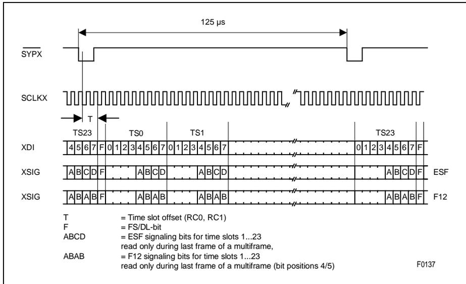
Figure 64 1.544 MHz Transmit Signaling Highway (T1/J1)
