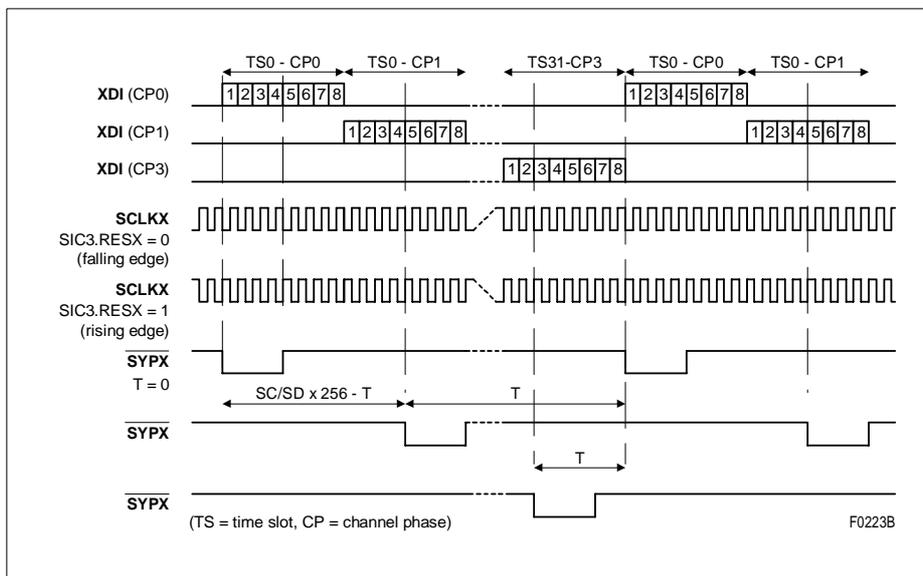
Figure 34 SYPX Offset Programming (8.192 Mbit/s, 8.192 MHz)
