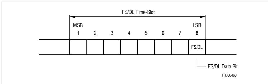
Figure 67 Transmit FS/DL Bits on XDI (T1/J1)
