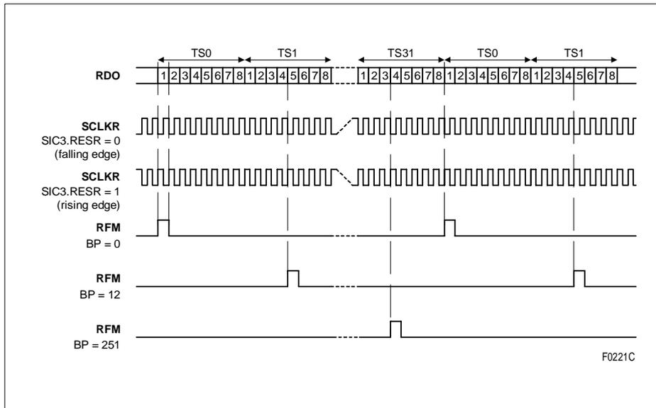
Figure 29 RFM Offset Programming (2.048 Mbit/s, 2.048 MHz)
