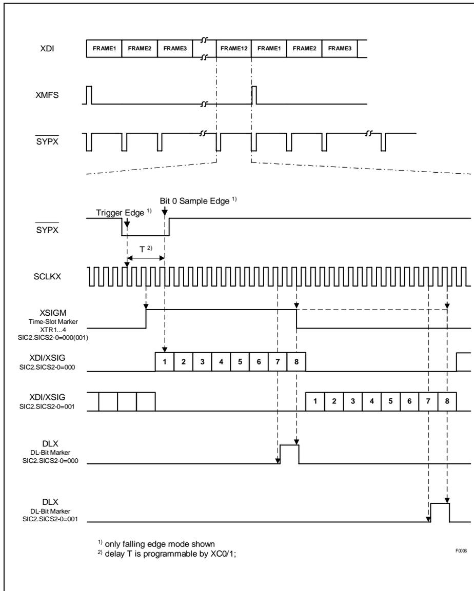
Figure 62 Transmit System Clocking: 8.192 MHz/4.096 Mbit/s (T1/J1)
