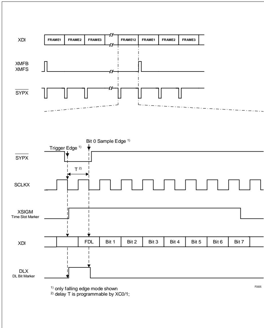
Figure 61 Transmit System Clocking: 1.544 MHz (T1/J1)
