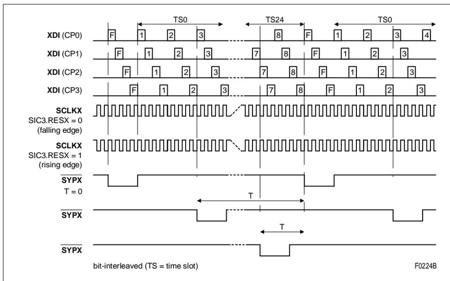
Figure 69 SYPX Offset Programming (6.176 Mbit/s, 6.176 MHz)
