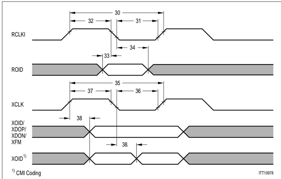
**Figure 88** Timing of Dual Rail Optical Interface
