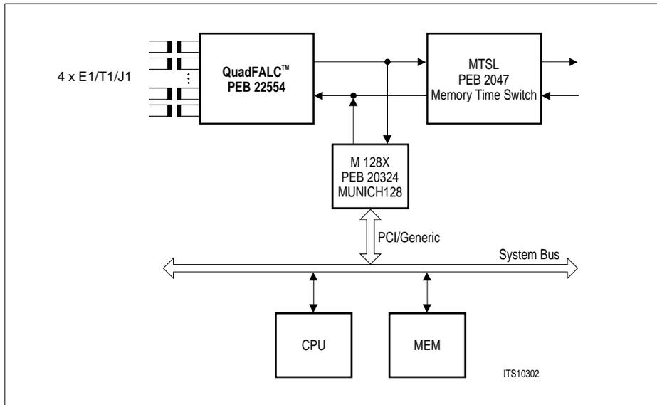
Figure 2 Multiple E1/T1/J1 Link over Frame Relay
