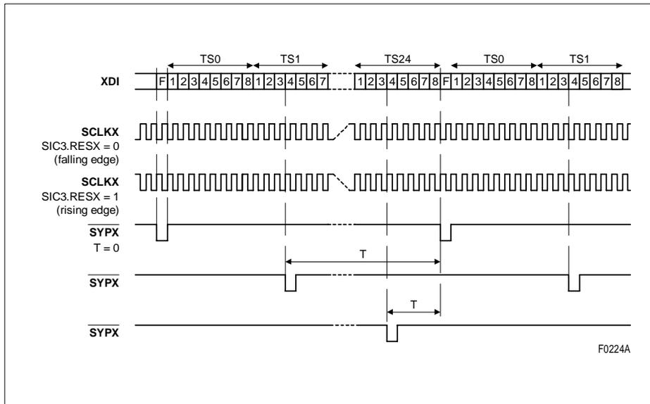
Figure 68 SYPX Offset Programming (1.544 Mbit/s, 1.544 MHz)
