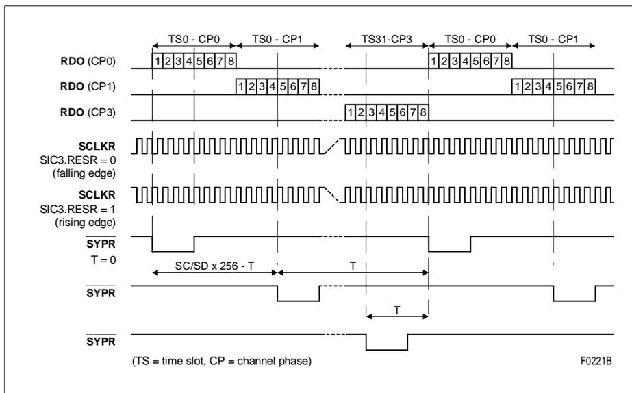
Figure 28 SYPR Offset Programming (8.192 Mbit/s, 8.192 MHz)
