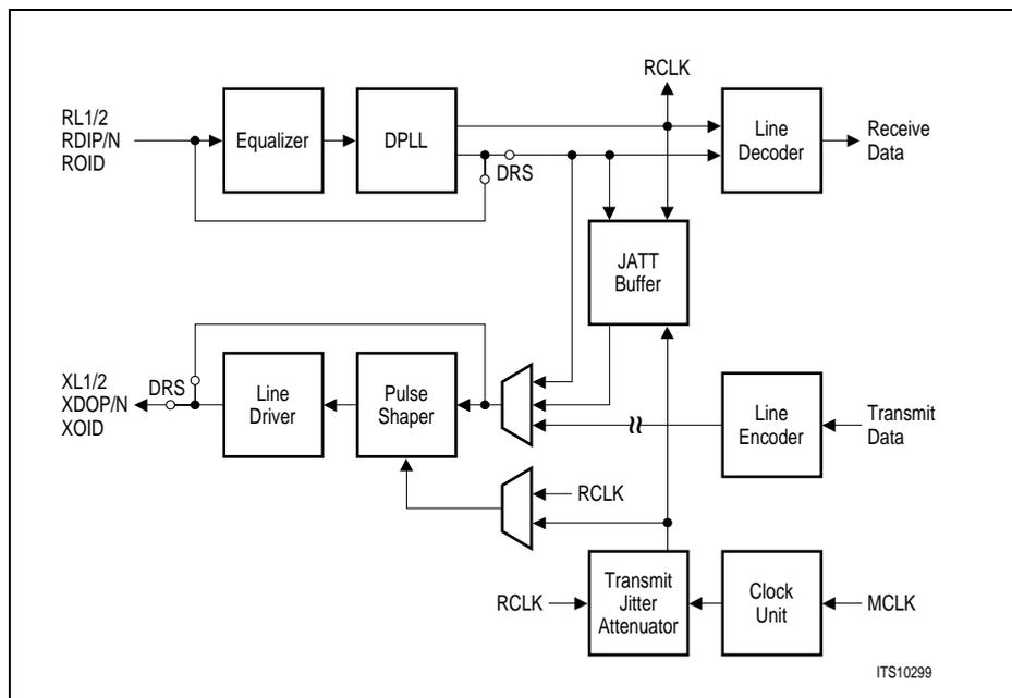
Figure 49 Clocking in Remote Loop Configuration (T1/J1)
