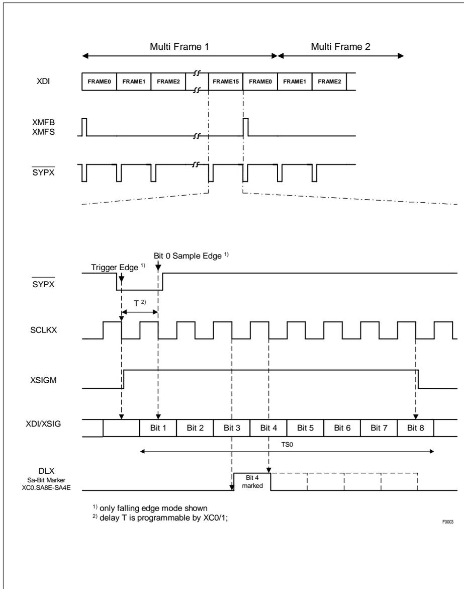
Figure 31 Transmit System Interface Clocking: 2.048 MHz (E1)
