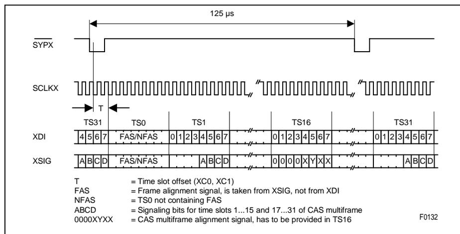
Figure 24 2.048 MHz Transmit Signaling Highway (E1)
