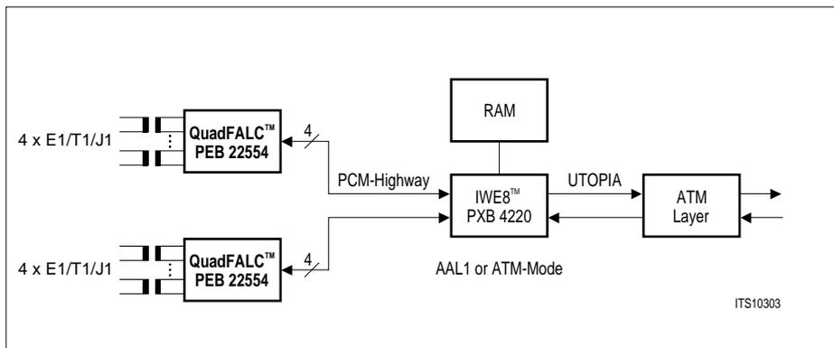
Figure 3 8 Channel E1/T1/J1 Interface to the ATM Layer
