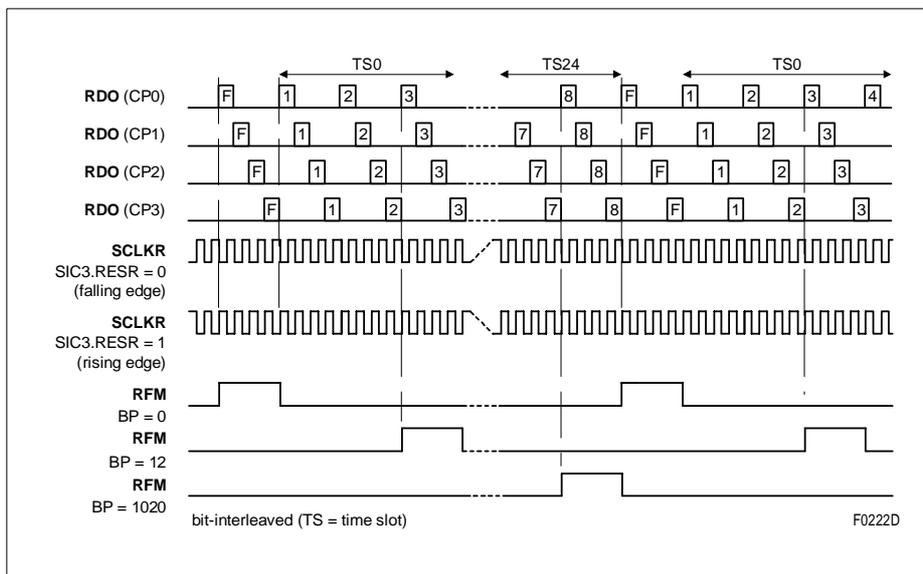
Figure 57 RFM Offset Programming (6.176 Mbit/s, 6.176 MHz)
