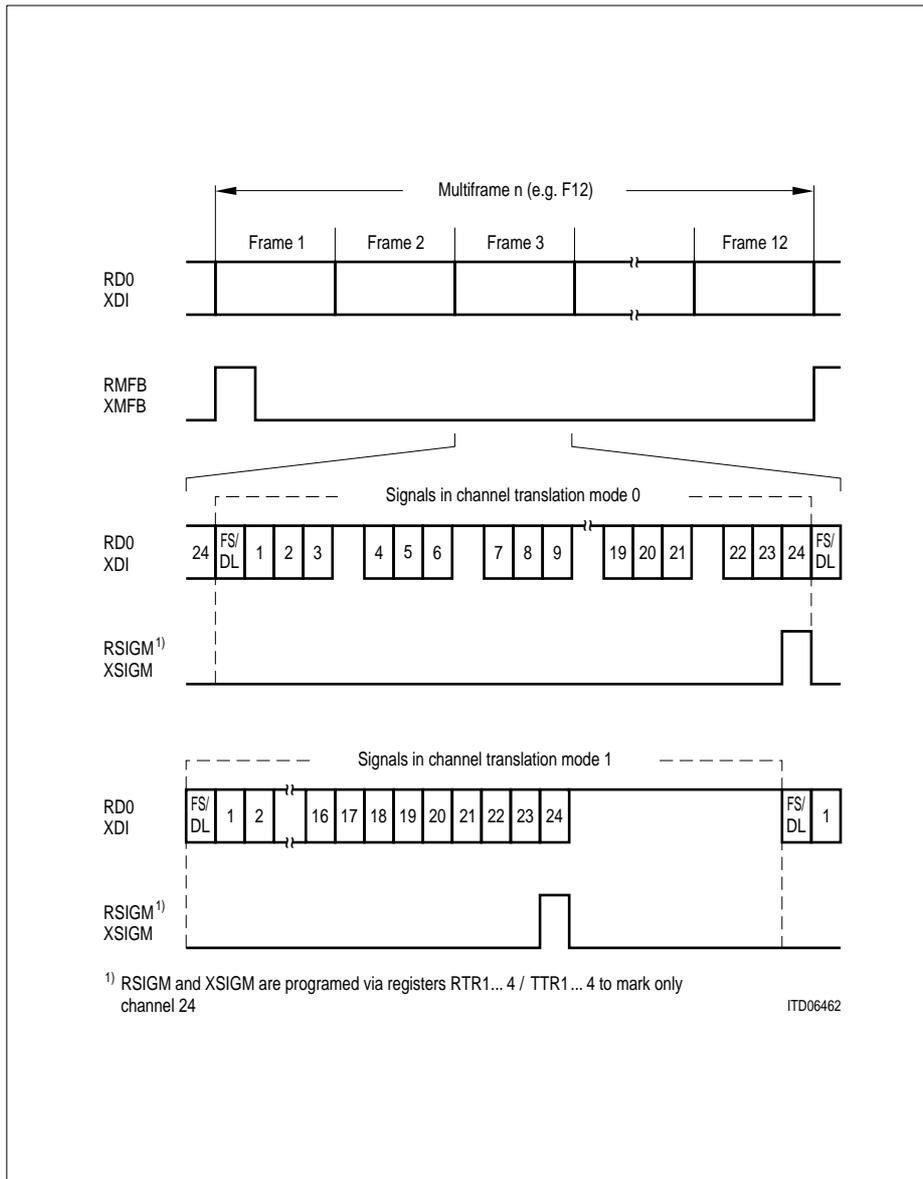
Figure 65 Signaling Marker for CAS/CAS-CC Applications (T1/J1)
