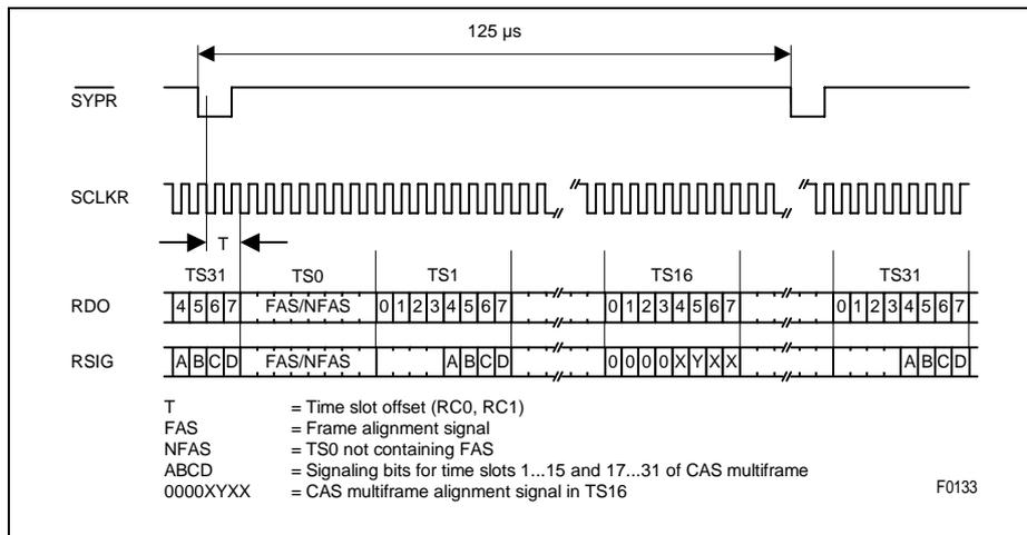
Figure 19 2.048 MHz Receive Signaling Highway (E1)
