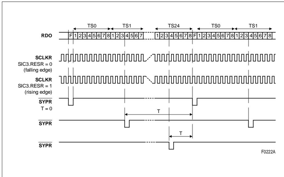
Figure 54 SYPR Offset Programming (1.544 Mbit/s, 1.544 MHz)
