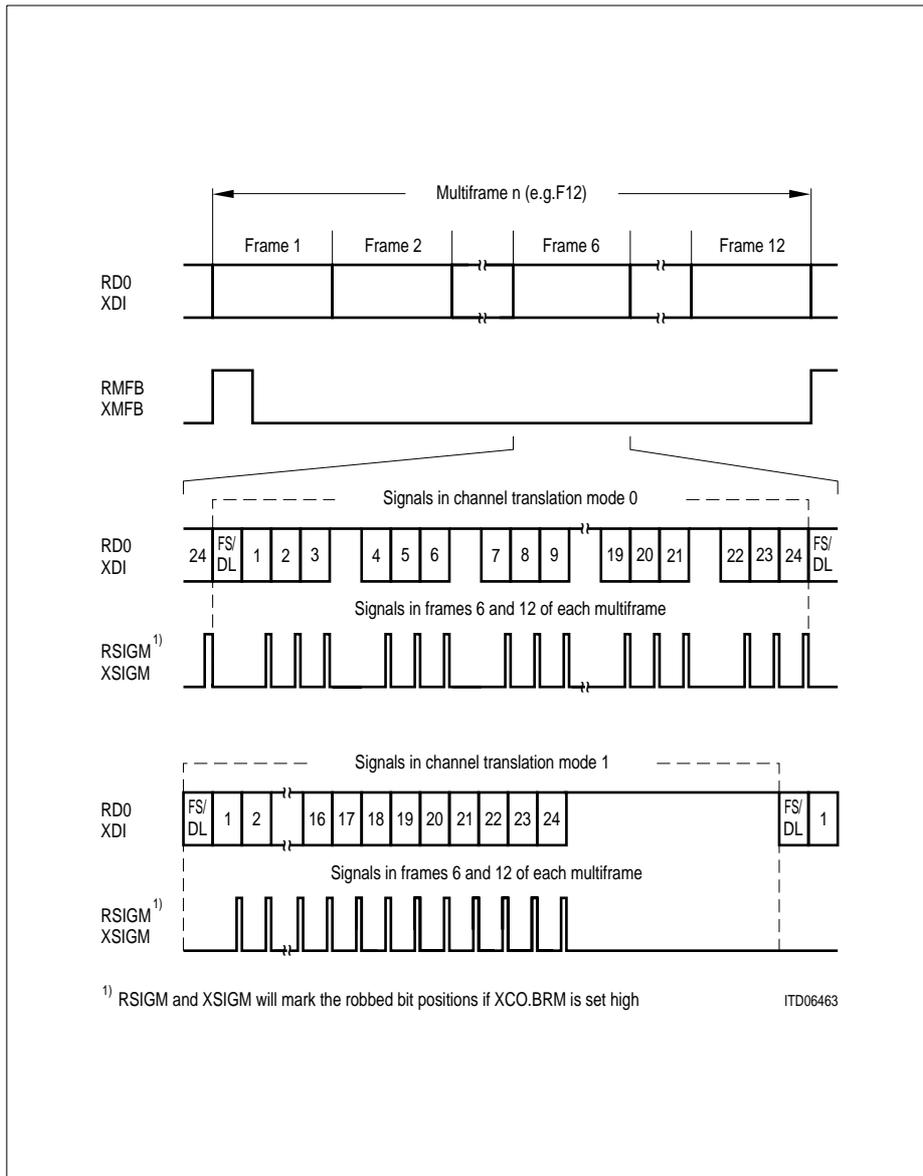
Figure 66 Signaling Marker for CAS-BR Applications (T1/J1)
