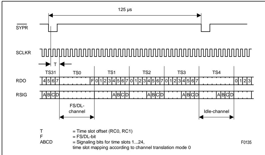
Figure 58 2.048 MHz Receive Signaling Highway (T1/J1)
