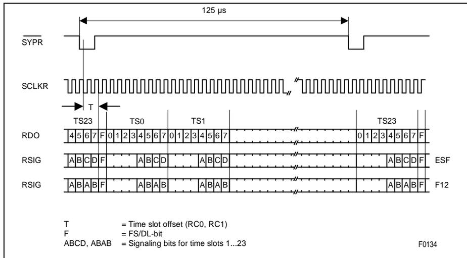
Figure 60 1.544 MHz Receive Signaling Highway (T1/J1)
