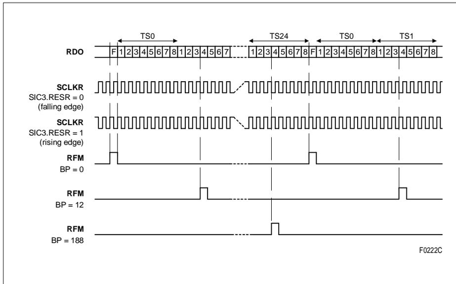
Figure 56 RFM Offset Programming (1.544 Mbit/s, 1.544 MHz)
