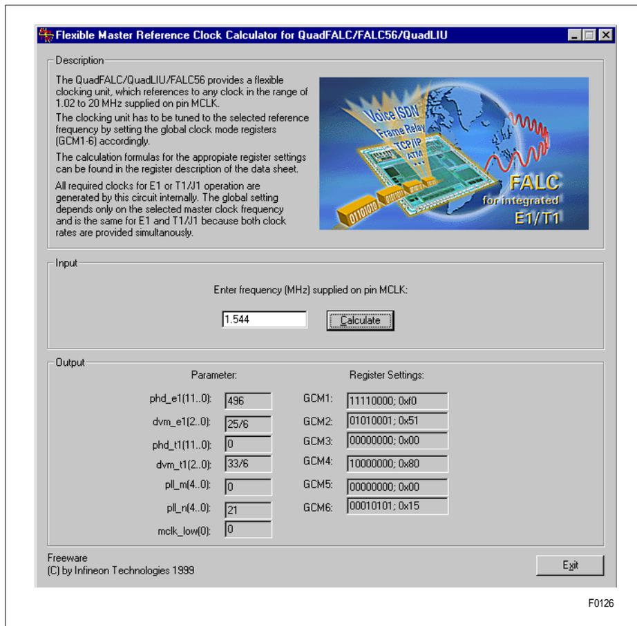
Figure 106 Master Clock Frequency Calculator
