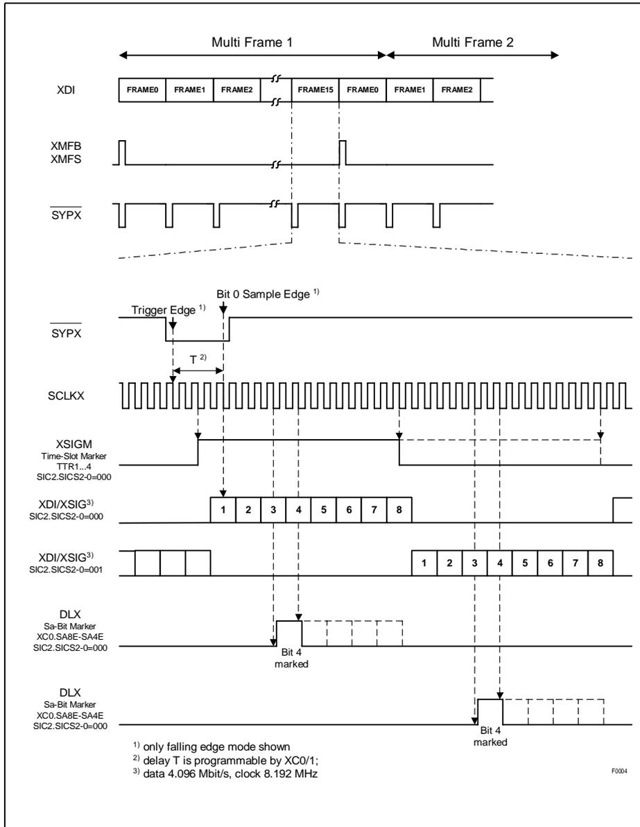
Figure 32 Transmit System Interface Clocking: 8.192 MHz/4.096 Mbit/s (E1)
