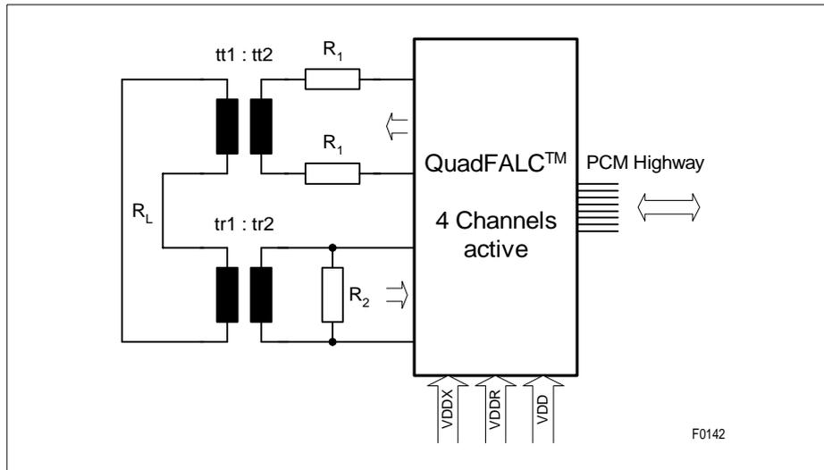
Figure 104 Device Configuration for Power Supply Testing
