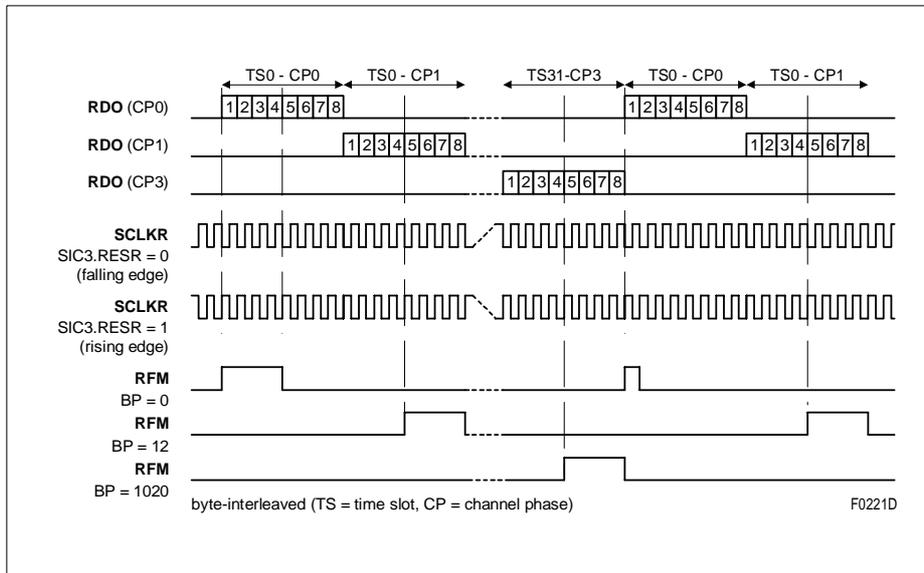
Figure 30 RFM Offset Programming (8.192 Mbit/s, 8.192 MHz)
