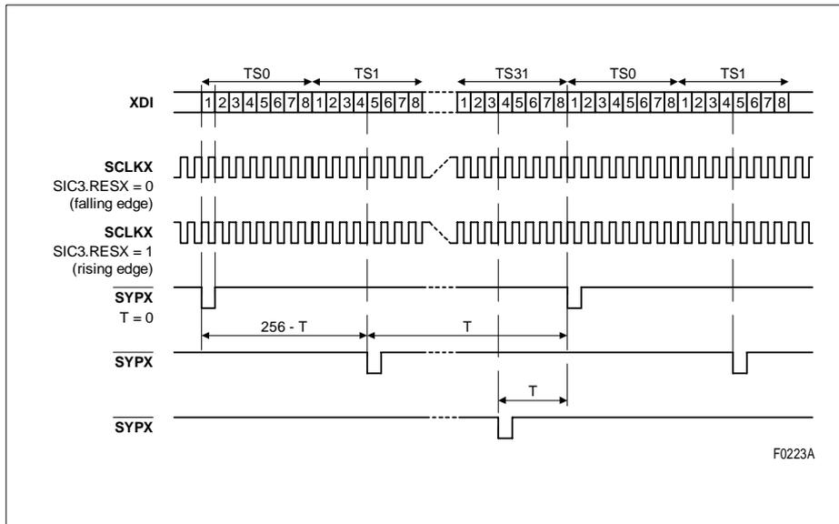
Figure 33 SYPX Offset Programming (2.048 Mbit/s, 2.048 MHz)
