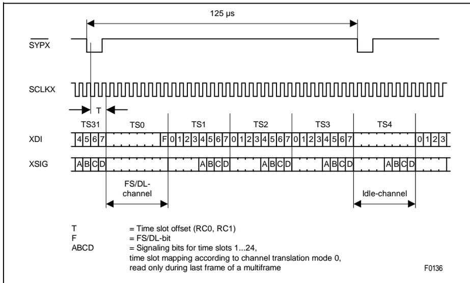
Figure 63 2.048 MHz Transmit Signaling Clcking (T1/J1)
