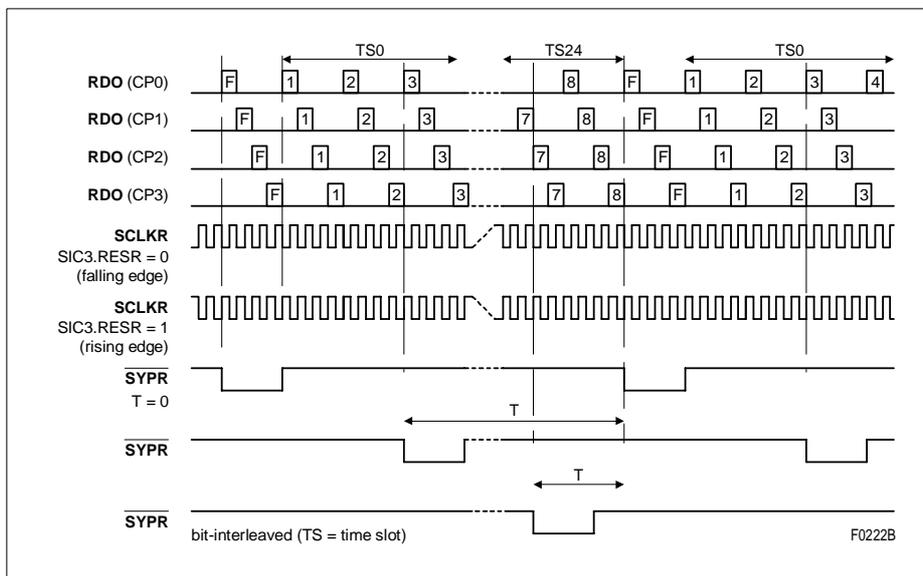
Figure 55 SYPR Offset Programming (6.176 Mbit/s, 6.176 MHz)
