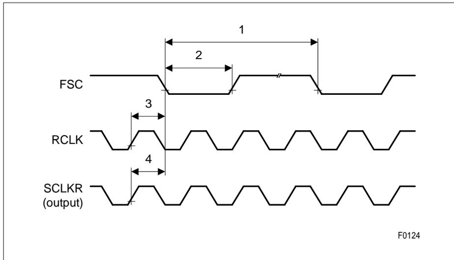
Figure 98 FSC Timing
