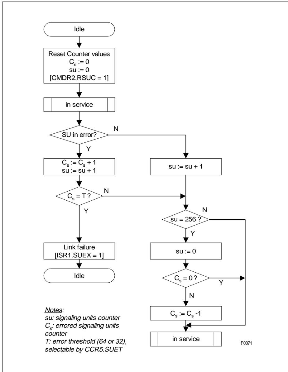
Figure 18 Automatic Handling of Errored Signaling Units
