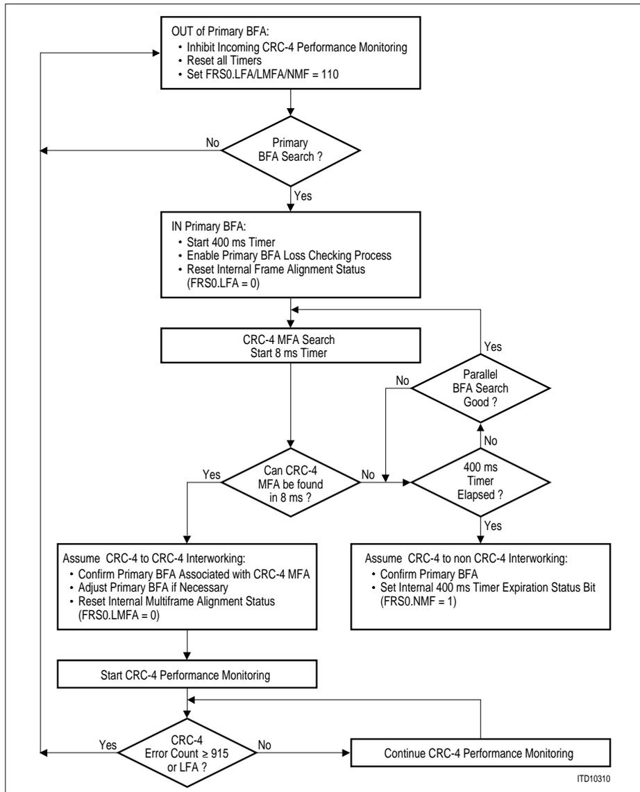
Figure 20 CRC4 Multiframe Alignment Recovery Algorithms (E1)
