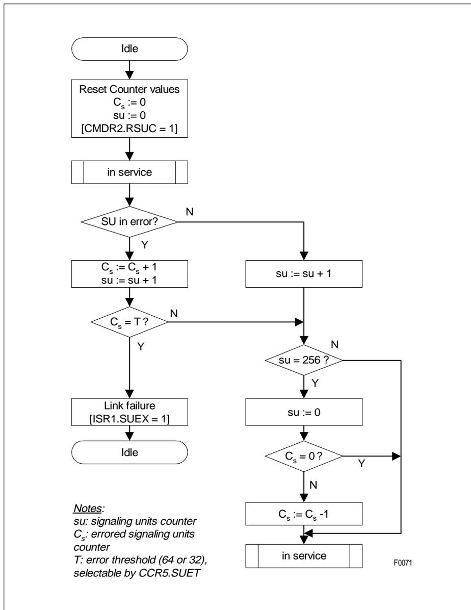
Figure 46 Automatic Handling of Errored Signaling Units
