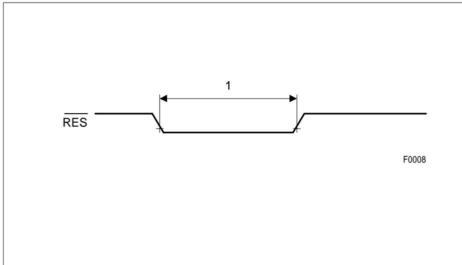
Figure 81 Reset Timing
