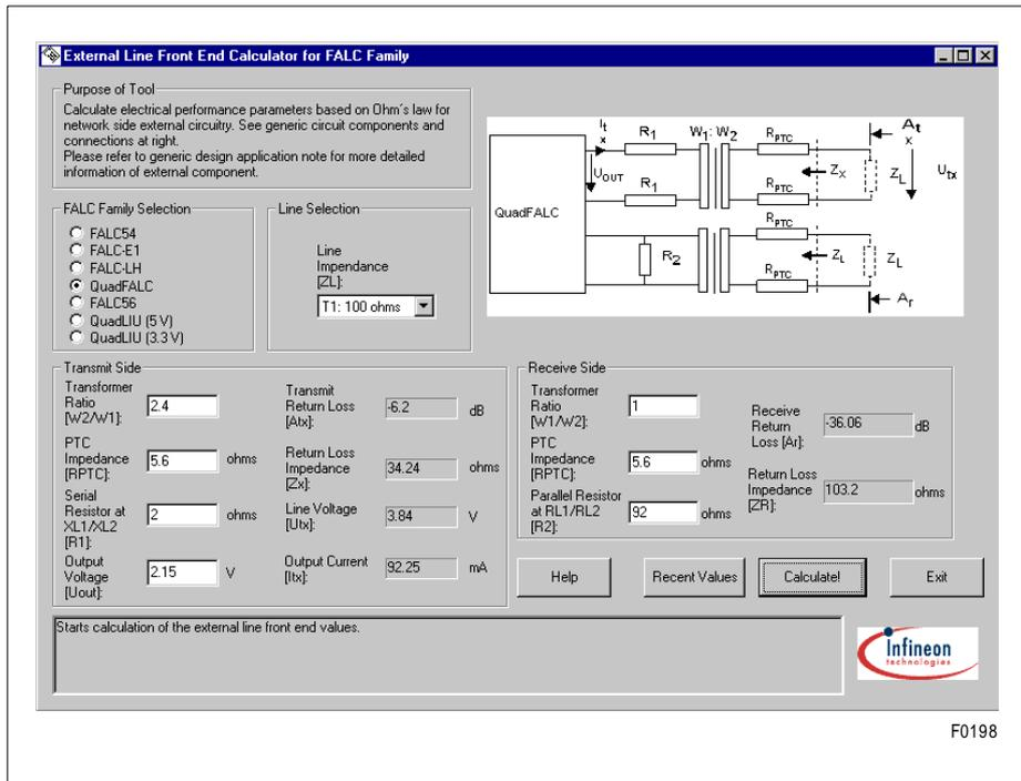
Figure 107 External Line Frontend Calculator
