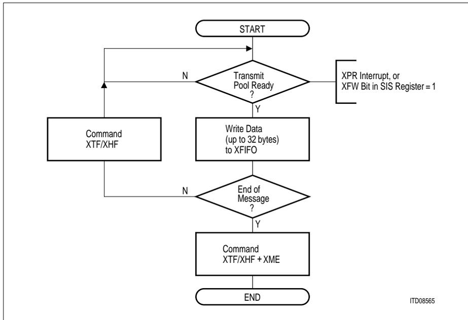
Figure 76 Interrupt Driven Data Transmission (flow diagram)
