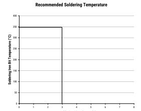
The soldering iron tip temperature should be set at 350°C (+10°C maximum) with the soldering duration not to exceed more than 3 seconds.
