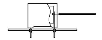
The temperature is monitored inside the capacitor.
