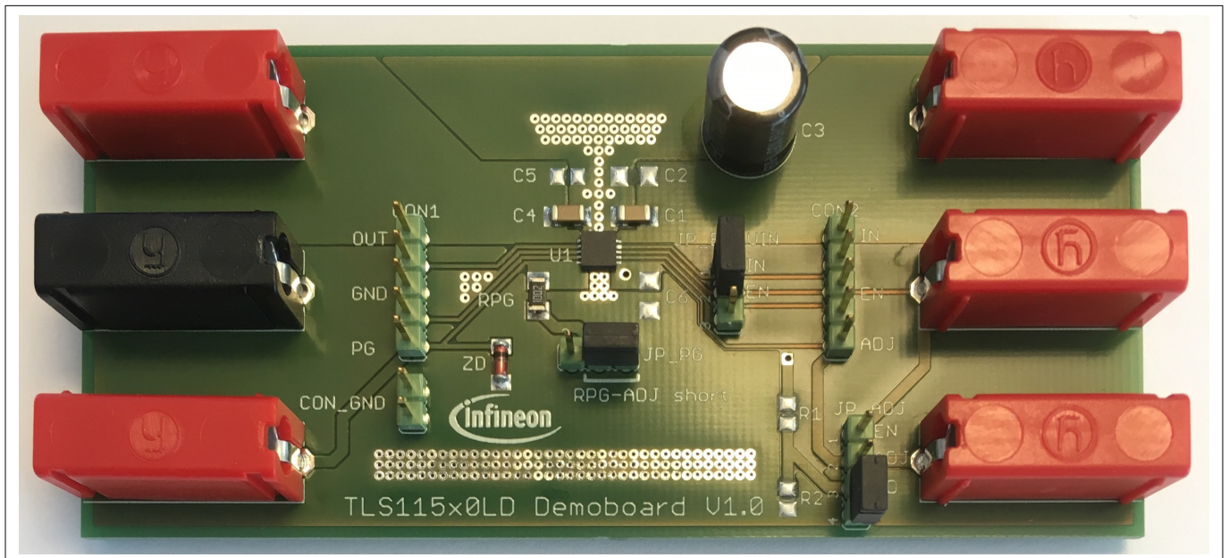
Figure 3 OPTIREG™ linear voltage regulator TLS115x0LD demoboard
