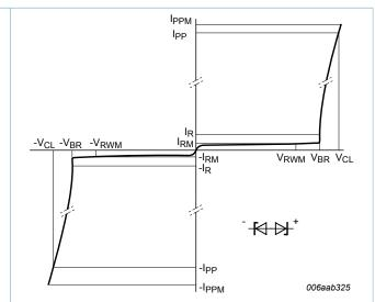
V-I characteristics for a bidirectional ESD protection diode
