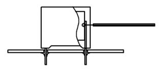
Temperature monitored inside the capacitor.
