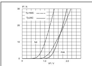
Fig.5. BY359X-1500 forward characteristic  $I_F = f(V_F)$ ; parameter  $T_j$
