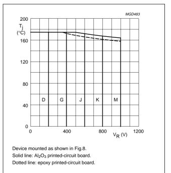
Fig.3 Maximum permissible junction temperature as a function of reverse voltage.
