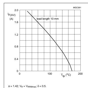
Fig.2 Maximum permissible average forward current as a function of tie-point temperature
