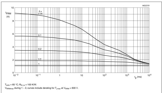
Fig.5 Maximum repetitive peak forward current as a function of pulse time (square pulse) and duty factor.
