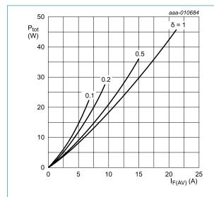
$I_{F(AV)} = I_{F(RMS)} \times \sqrt{\delta}$   $V_0 = 1.578; R_s = 0.027 \Omega$
