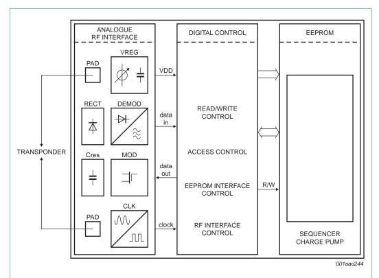
Fig 1. Block diagram of HITAG 2 transponder IC
