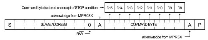
Figure 10. Command Byte Received
