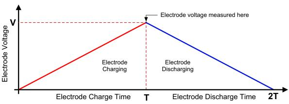
Figure 21. MPR03X Electrode Measurement Charging Pad Capacitance
