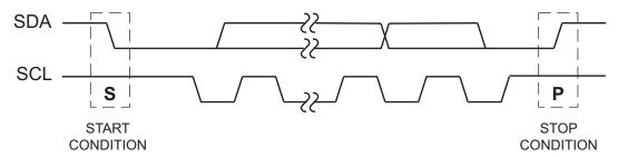
Figure 7. Stop and Start Conditions
