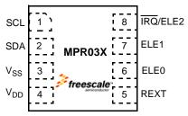
Figure 3. Package Pinouts
