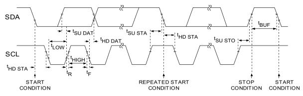
Figure 5. Wire Serial Interface Timing Details
