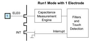
Figure 14. Electrode/Pad Connections in Run Mode
