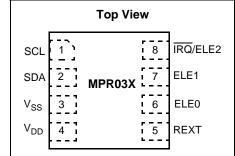
Figure 1. Pin Connections
