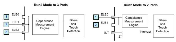
Figure 15. Electrode/Pad Connections in Area Detection Mode
