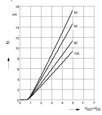
**Drain current**  $I_D = f(V_{GG})$  amp. B  $V_{DS} = 5V$ ,  $V_{G2S} = 4V$ ,  $R_{G1} = 50k\Omega$ (connected to  $V_{GG}$ ,  $V_{GG}$ =gate1 supply voltage)
