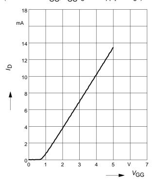
Drain current  $I_D = f(V_{GG})$  $V_{G2S} = 4V$ ,  $R_{G1}$  = Parameter in kΩ amp. B
