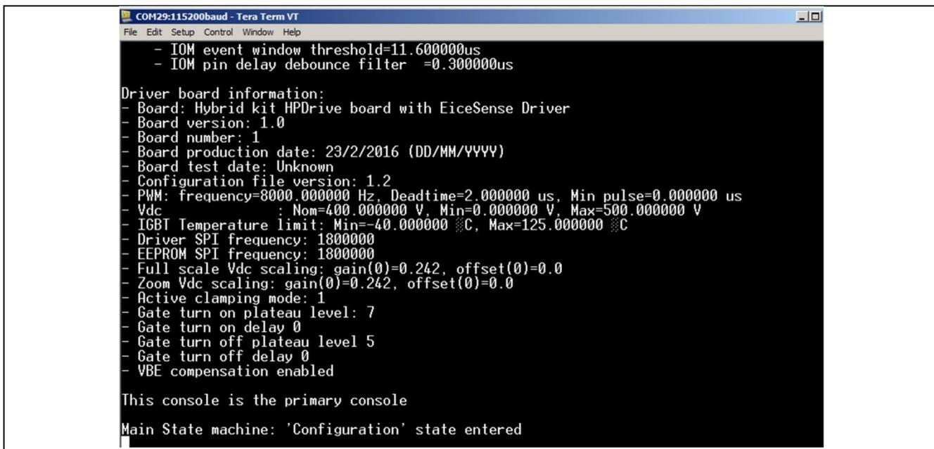
**Figure 6** Typical appearance, when terminal program is connected right and evaluation kit was power toggled. The evaluation kit enters automatically the “Configuration State” (please ensure that DEMO-ENABLE-PLUG is not connected).
