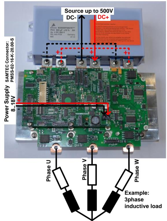
Figure 1 HybridKIT Drive typical appearance and connections.
