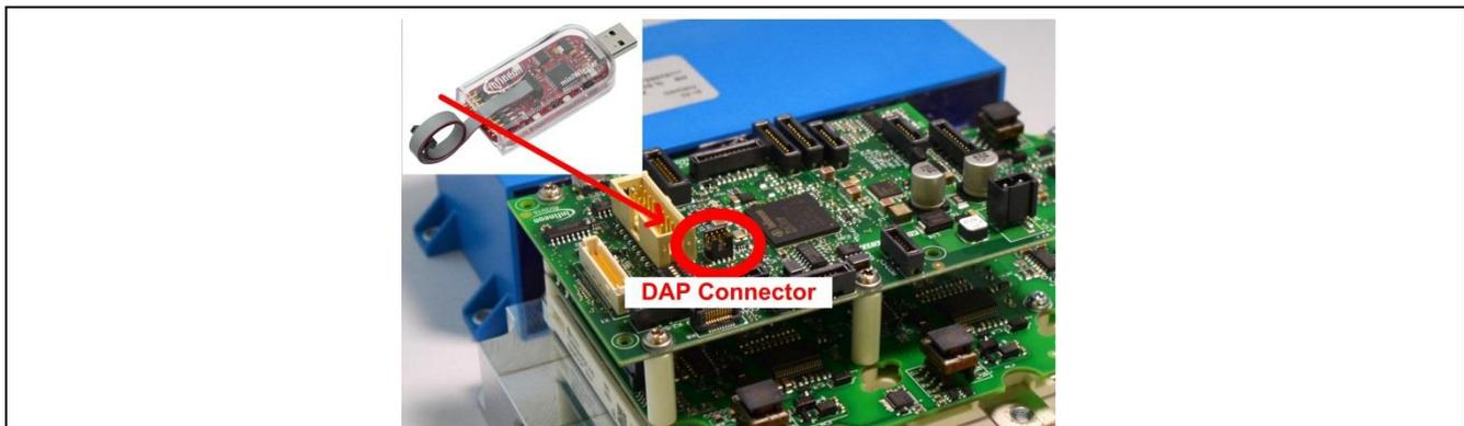
Figure 3 DAP miniWiggler and connector typical position on the evaluation kit.
