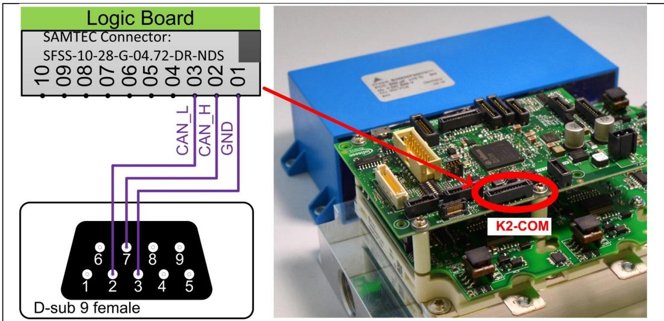
Figure 10 Example for connecting via CAN bus communication.
