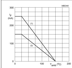
Device mounted on an FR4 printed-circuit board.
