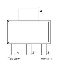
Fig.1 Simplified outline (SOT223) and pin configuration.
