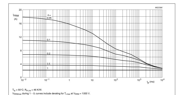
Fig.4 Maximum repetitive peak forward current as a function of pulse time (square pulse) and duty factor.
