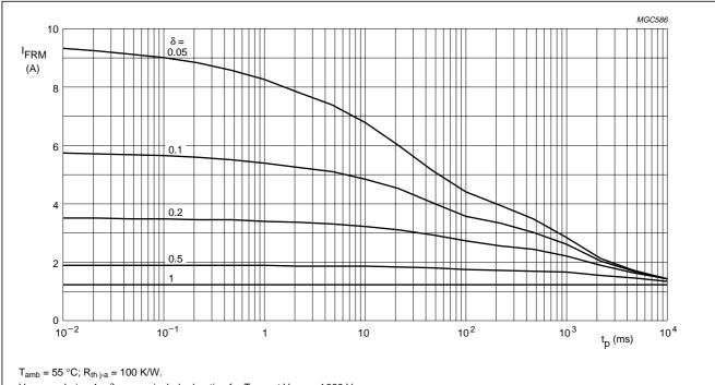
$V_{RRMmax}$  during 1 –  $\delta$ ; curves include derating for  $T_{j\,max}$  at  $V_{RRM}$  = 1000 V.
