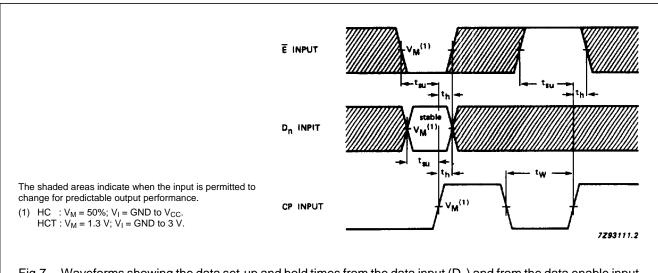
Fig.7 Waveforms showing the data set-up and hold times from the data input  $(D_n)$  and from the data enable input  $(\overline{E})$  to the clock (CP).
