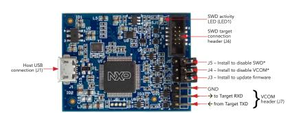
\*J4 and J5 jumper headers may not be installed on all boards.
