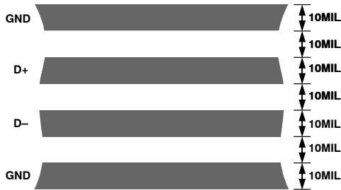
Figure 19. Arrangement of Signal Tracks
