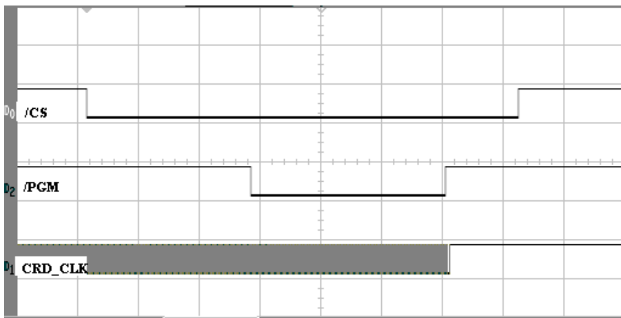
Figure 29. Clock Divider: Run to Stop High Operation
