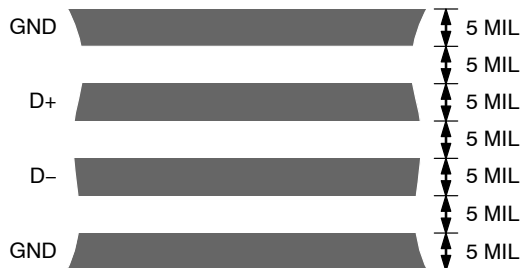
Figure 22. Typical Arrangement of Signal Tracks
