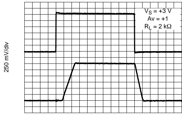
Figure 24. 3 V Non-Inverting Large Signal Pulse Response
