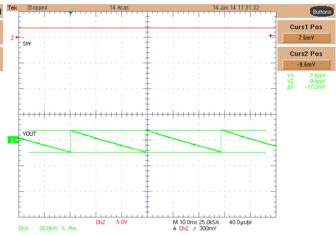
Figure 15. DCDC2 Ripple Voltage in PFM Mode ( V_{IN} = 3.6\text{ V} - V_{OUT} = 1.8\text{ V} - \text{No load} )
