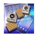
The NCP6924 is part of the ON Semiconductor mini-power management IC family. It is optimized to supply battery powered portable application subsystems such as camera modules, microprocessors or any peripherals. This device integrates two high efficiency 1000 mA step-down DC to DC converters with DVS (Dynamic Voltage Scaling) and four low dropout (LDO) voltage regulators in WLCSP-30 2.46 x 2.06mm package.
