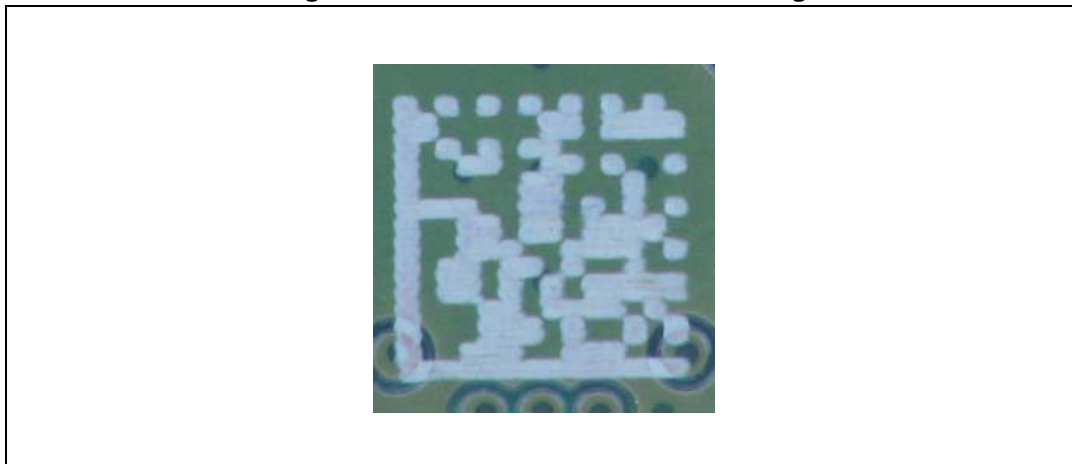
Figure 8. SPSGRF QR-code laser marking
