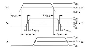
$t_{PHL1}$  and  $t_{PLH1}$  are the  $t_{PHL}$  and  $t_{PLH}$ , respectively, for the output under test, Om.  $t_{PHL2}$  and  $t_{PLH2}$  are the  $t_{PHL}$  and  $t_{PLH}$ , respectively, for any other output, On. Where m = 0 to 7, n = 0 to 7, and m is not equal to n.
