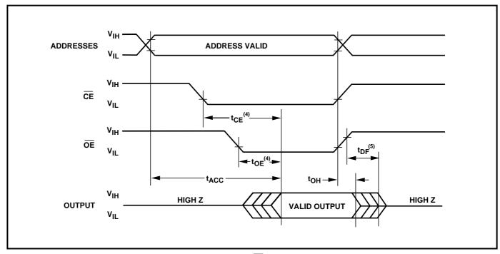
**NOTE:** 4.  $\overline{OE}$  may be delayed up to  $t_{CE} - t_{OE}$  after the falling edge of  $\overline{CE}$  without impact on  $t_{CE}$ .
