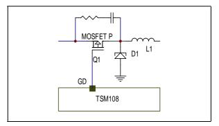
The RC components should realise a time constant corresponding to one tenth of the switching time constant of the TSM108 (i.e. in our example, the oscillator frequency is set to 10 $\mu$ s corresponding to 100kHz, therefore, the RC couple should realise a time constant close to 1 $\mu$ s).
