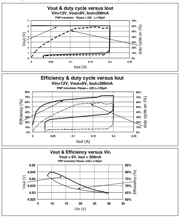
12.2. Voltage and Current Control, Efficiency Performances using a PNP bipolar transistor
