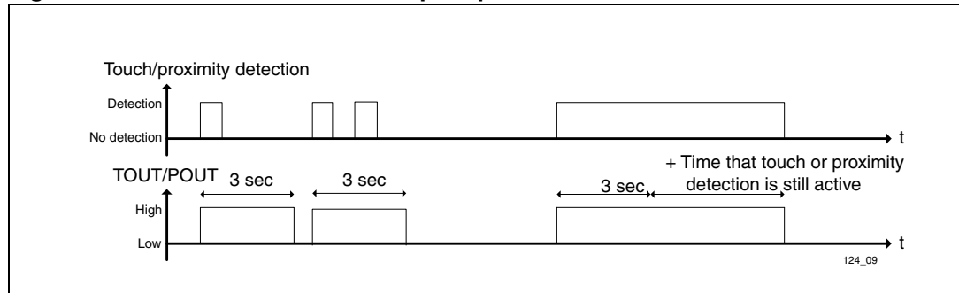
Figure 14. 3-second latch mode output operation
