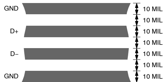
Figure 17. Arrangement of Signal Tracks
